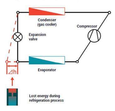
The ejector achieves this by increasing the compressor's intake pressure. Sounds complicated, right? The essential point is that ejectors yield significant long-term cost benefits to end users.
