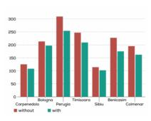
The data produced by the systems during the 3 years of observation were processed as part of a precise consumption analysis, demonstrating that the Epta technologies used in the Life-C4R guarantee an annual decrease in energy consumption of between 15% and 23% (compared to traditional CO<sub>2</sub> systems).
